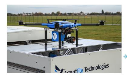
The drone can be equipped with various EO/IR payloads and additional onboard electronics, like an e-ident device, ADS-B transponder, or antijamming/antispoofing modules for operation in a harsh environment.
